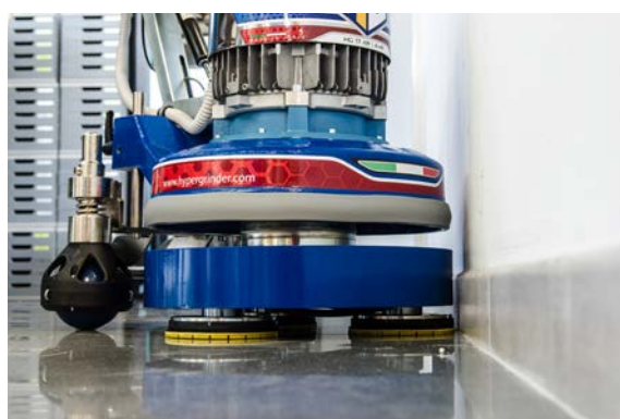
Ideal machine for grinding flush against walls.
